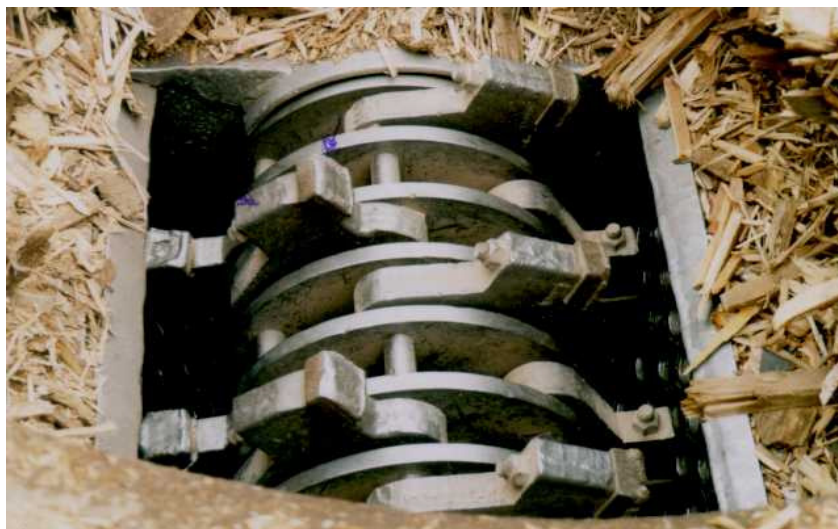
Fig. 4. Wood crusher as example for repair based maintenance
