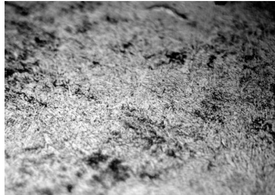
Fig. 6. Tempered hardening steel, t_{max} = 800\text{ }^{\circ}\text{C} , \Delta\varepsilon=0.8\% , N=136 cycles; structure in test piece tensile zone (x 1000)
