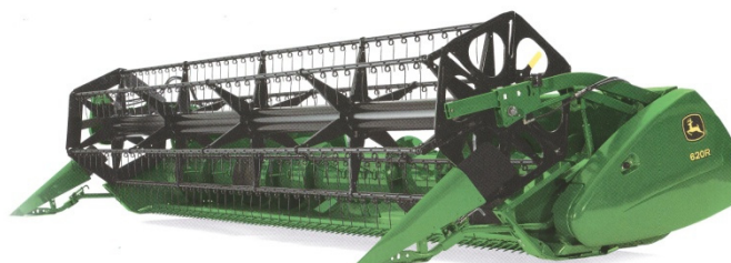
Fig. 1: Illustration of a wheat adapter (header)
