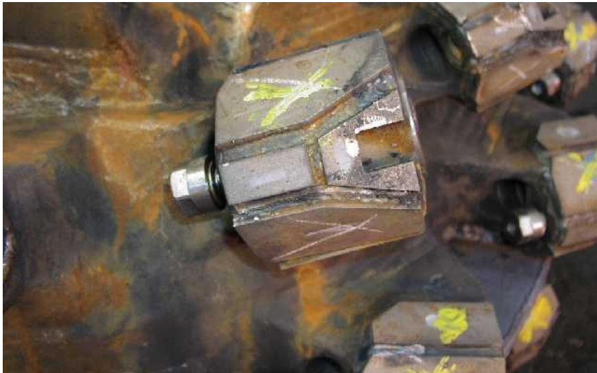
Fig. 7. Tool holder with wear protection plates made of NiCrBSi coated mild steel.
