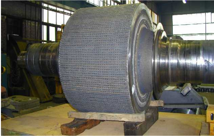
Fig. 5. Crusher roll for clinker preventively wearfaced by welding with flux cored wires in different grades to get a gradient of hardness and wear resistance.
