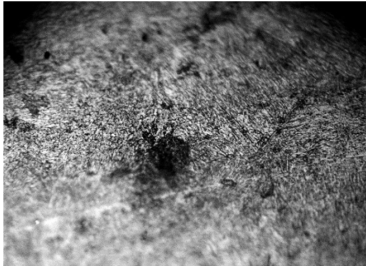
Fig. 5. Tempered hardening steel, t_{max} = 800\text{ }^{\circ}\text{C} , \Delta\varepsilon=0.8\% , N=136 cycles; structure in test piece central zone (x 1000)
