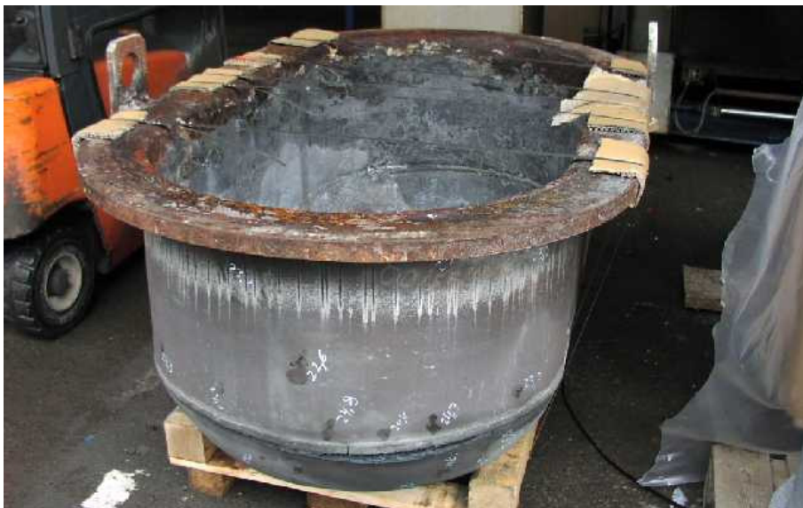
Fig. 6. Melting pot for potassium permanently under visual control to achieve maximum lifetime
