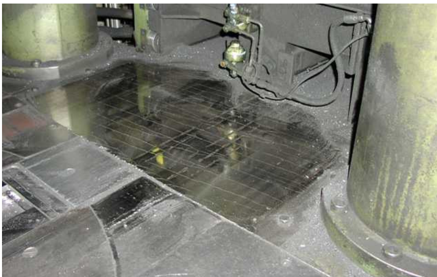
Fig. 8. Machined wearplate for filling the die with raw materials for fireclay.
